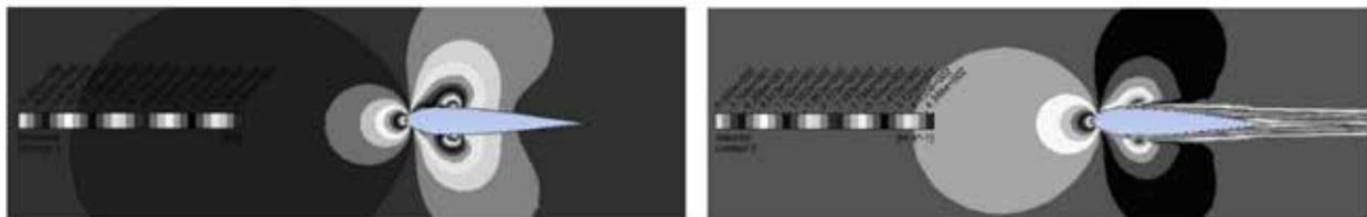
Fig. 5. Design 3 pressure (top) and velocity (below) contour at 0°.
