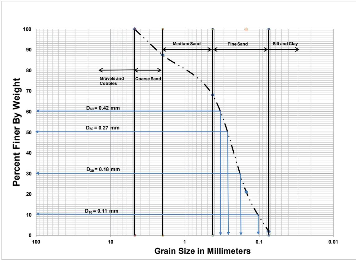
Fig. 3. Grainsize analysis of the soil sample.
