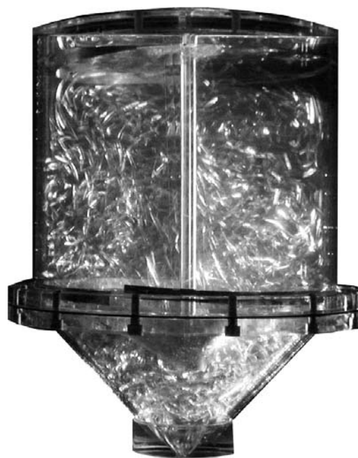
Fig. 2. Flow visualization performed in the conical vessel with a retreat curve impeller and a single wall baffle (located behind the impeller shaft).
