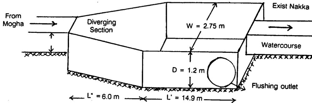
Fig. 4. Designed settling basin with automatic flushing.
