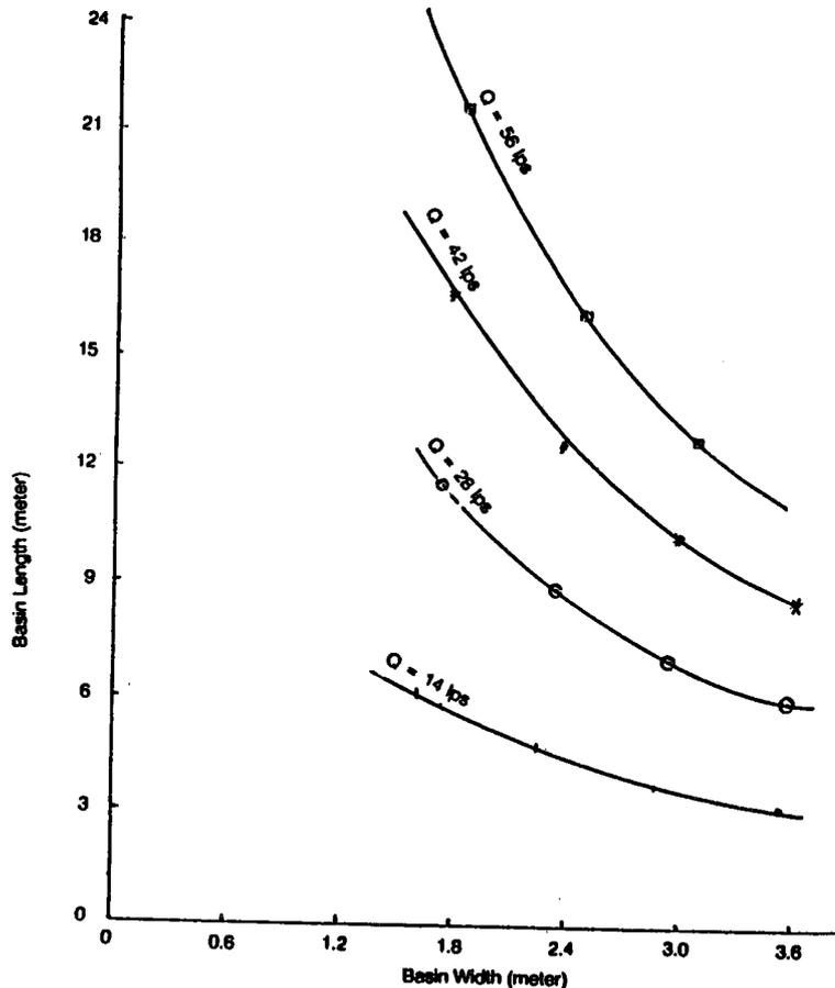
Fig. 2. Basin length as affected by width for various discharge values.
