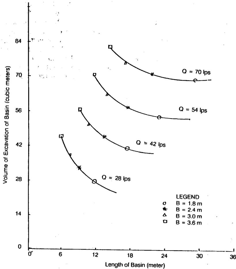
Fig. 3. Volume of excavation as affected by the width of basin.
