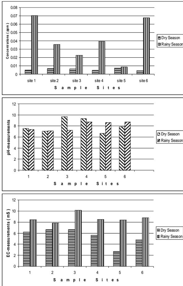
Figure 1. Comparison of Cd concentrations (ppm) of Contaminated Water Samples with Relation to the pH and EC-values of the same sites in Khartoum Industrial area
