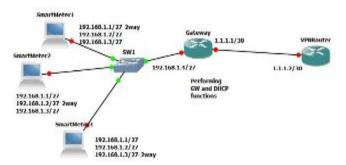
random manner, such that the IP address used by the same client varies each time while communicating. However for making two way communication possible using such method, there must be some device in between which has a track of the MAC to IP binding and the NAT sessions.
