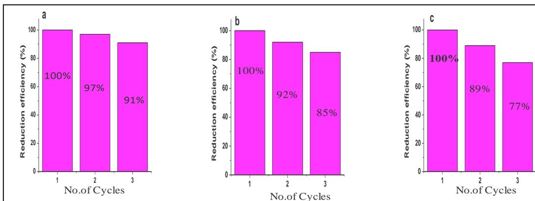
Figure 8. Percent reduction potential of glass supported Ge-AuNPs recovered and re-used for 3 successive cycles (a) EB (b) MB (c) RB.
