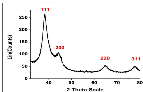
Figure 4. X-Ray diffraction (XRD) pattern showing Gel-AuNPs.
