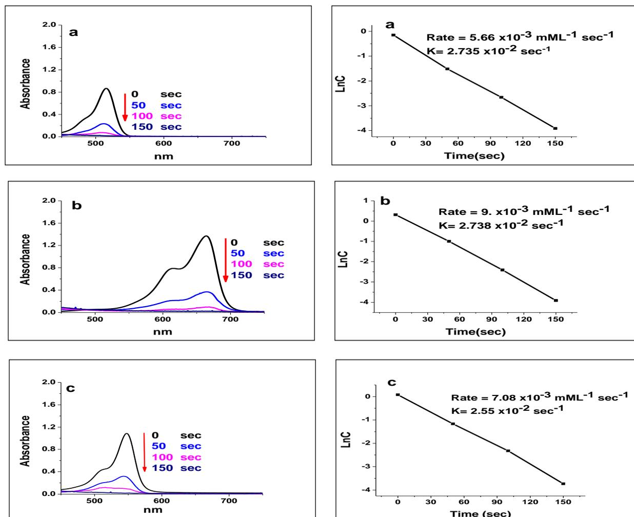
Figure 7. (a) Plot of lnC Vs Time (sec) showing first order kinetics at 10 μM of each dye (a) EB (b) MB (c) RB reduction using Gel-AuNPs as catalyst.
