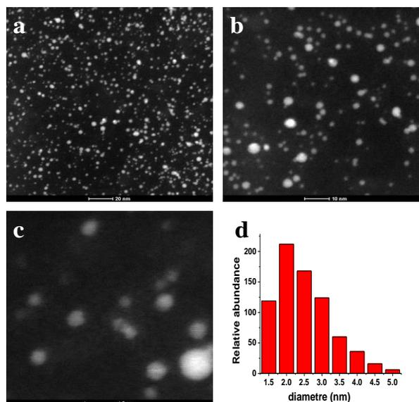
Figure 2. (a-b) STEM micrograph showing gel-AuNPs at different magnifications and corresponding size distribution histogram of Gel-AuNPs (Fig. 2a).
