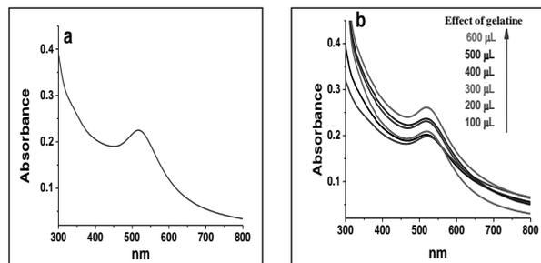
Figure 1. (a) Showing Surface plasmon resonance band of Gel-AuNPs (b) Effect of different concentration 0.5% gelatin.
