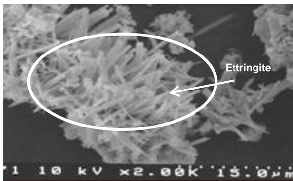
Figure 1. Ettringite observed in the dried products after the coagulation.
