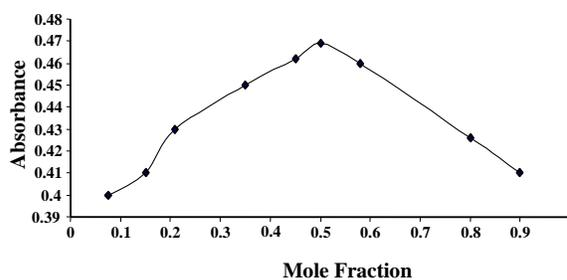
Figure 3. Job's plot for  $\text{Hg}^{2+}$  complex of ligand **3**.
