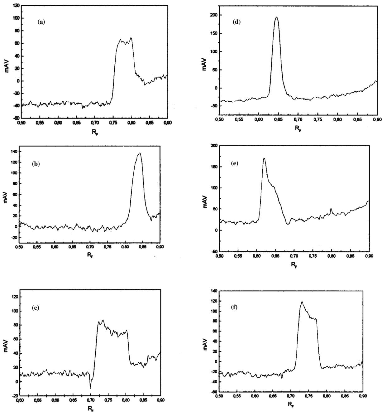
Figure 3. Sequence of the densitometric concentration profiles of S,R-(±)-2-phenylpropionic acid after: (a) 0 h; (b) 22.5 h; (c) 27.5 h; (d) 46.5 h; (e) 51.5 h; and (f) 70.5 h storage time in 70% ethanol at  $22 \pm 2^\circ\text{C}$ . Changes of the concentration profiles are accompanied by the changing  $R_F$  values (originally published in [7])
