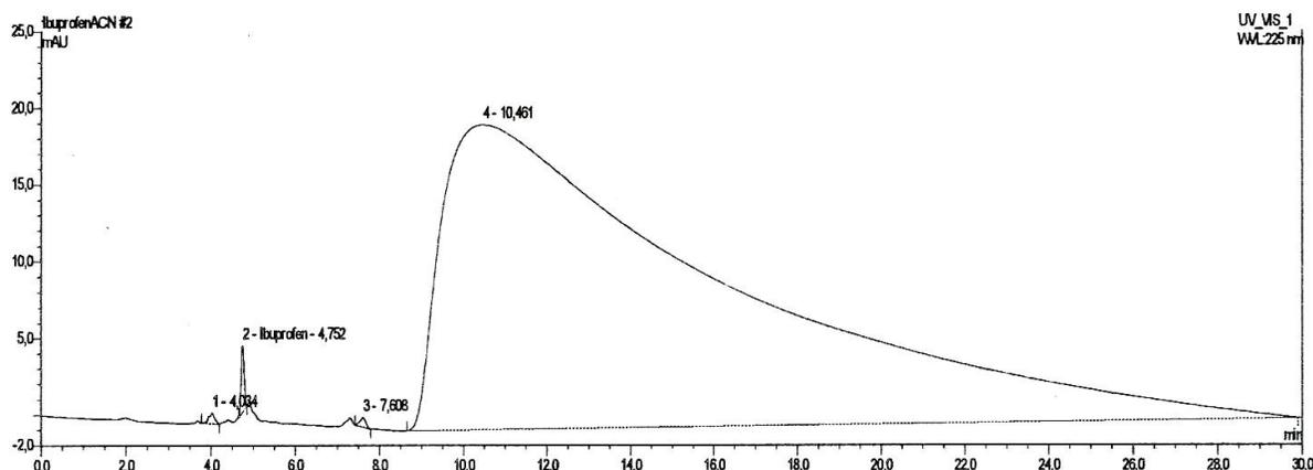
Figure 7. The tailing concentration profile on the high performance liquid chromatogram of S-(+)-ibuprofen dissolved in acetonitrile and chromatographed in the RP-18 / acetonitrile HPLC system at ambient temperature (originally published in [20])
