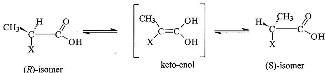
Scheme 1. The mechanism of transenantiomerization of 2-APAs via the keto-enol tautomerism (X: aryl substituent of propionic acid in position 2 of the carbon chain)
