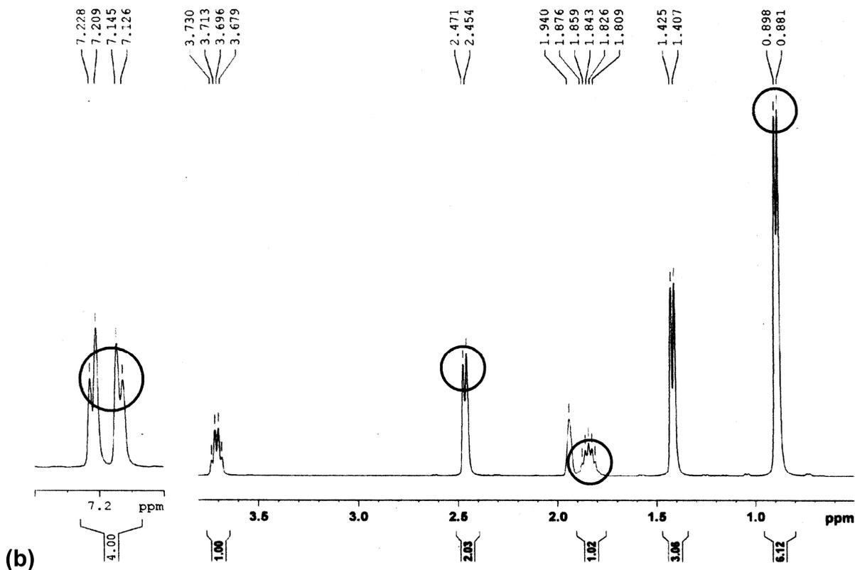
Figure 8. The  $^1\text{H}$  NMR spectra of S-(+)-ibuprofen dissolved in  $\text{ACN-D}_3$  and recorded with use of (a) the rotating probe and (b) the non-rotating probe. With circles these particular spectral regions were marked, for which recording in a rotating probe came out particularly inaccurate, i.e., the split of the respective signals was incomplete (originally published in [20])
