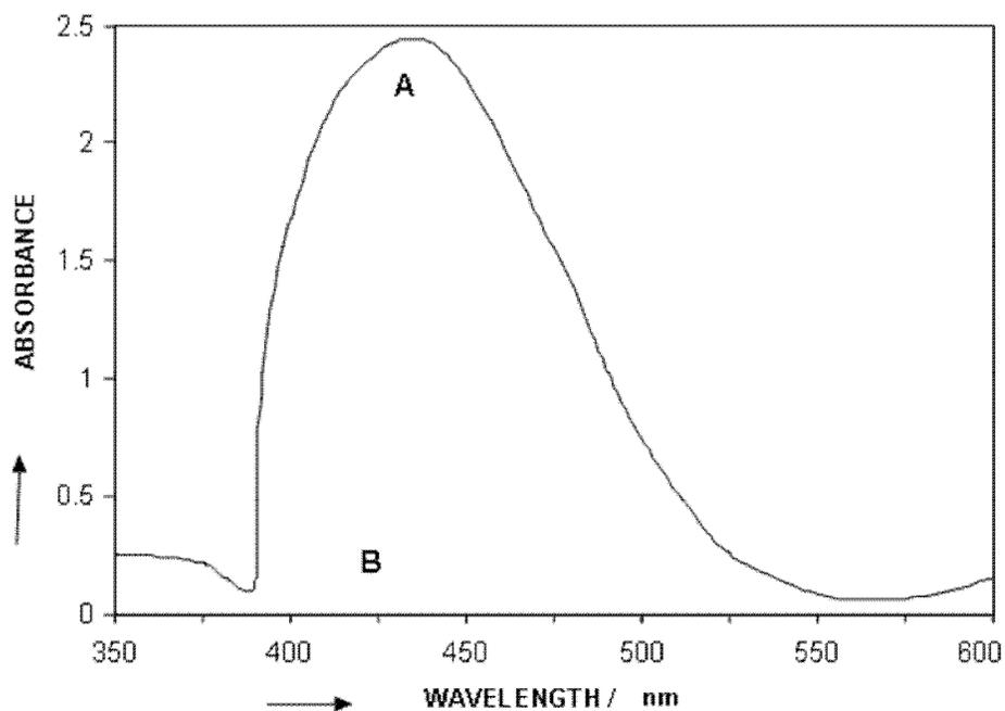
Fig. 1. A and B absorption spectra of molybdenum-HAPBH and the reagent blank ( $\lambda_{\max} = 443$  nm) in aqueous solution
