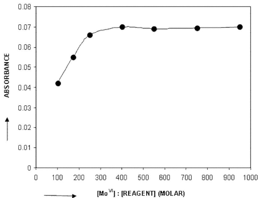
Fig. 3. Effect of reagent on the absorbance of Mo<sup>VI</sup>-HAPBH system.
