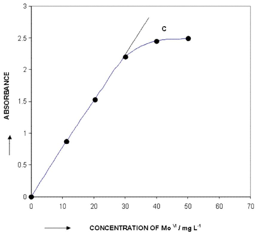
Fig. 4. Calibration graph C:10-30 mg L<sup>-1</sup> of molybdenum(VI)
