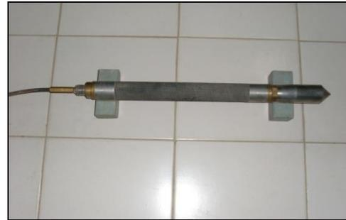
**Fig. 1 The Akbar Pressuremeter**
