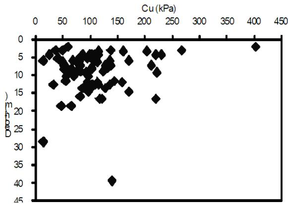
**Figure 1:** Variation of un-drained cohesion ( $C_u$ ) with depth at the project site.
