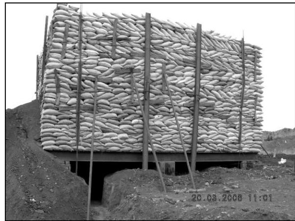
**Plate 1:** A view of soil filled bags on loading platform to obtain dead load reaction
